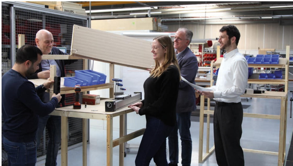
During the LEAN solutions workshops, the team develops a wood and cardboard model of the future workstation.
